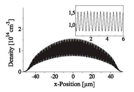
condensate density profile in a lattice potential + harmonic confinement
