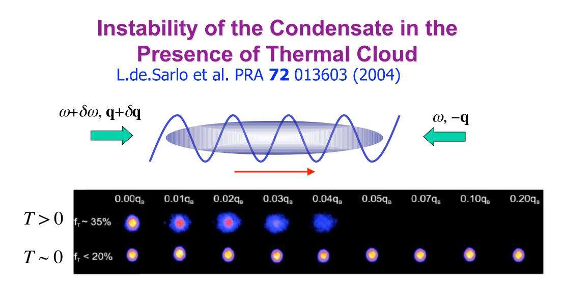
In the presence of the thermal cloud, one observes a strong reduction of the condensate atoms, even when the lattice velocity is well below the critical velocity for the dynamical instability.
