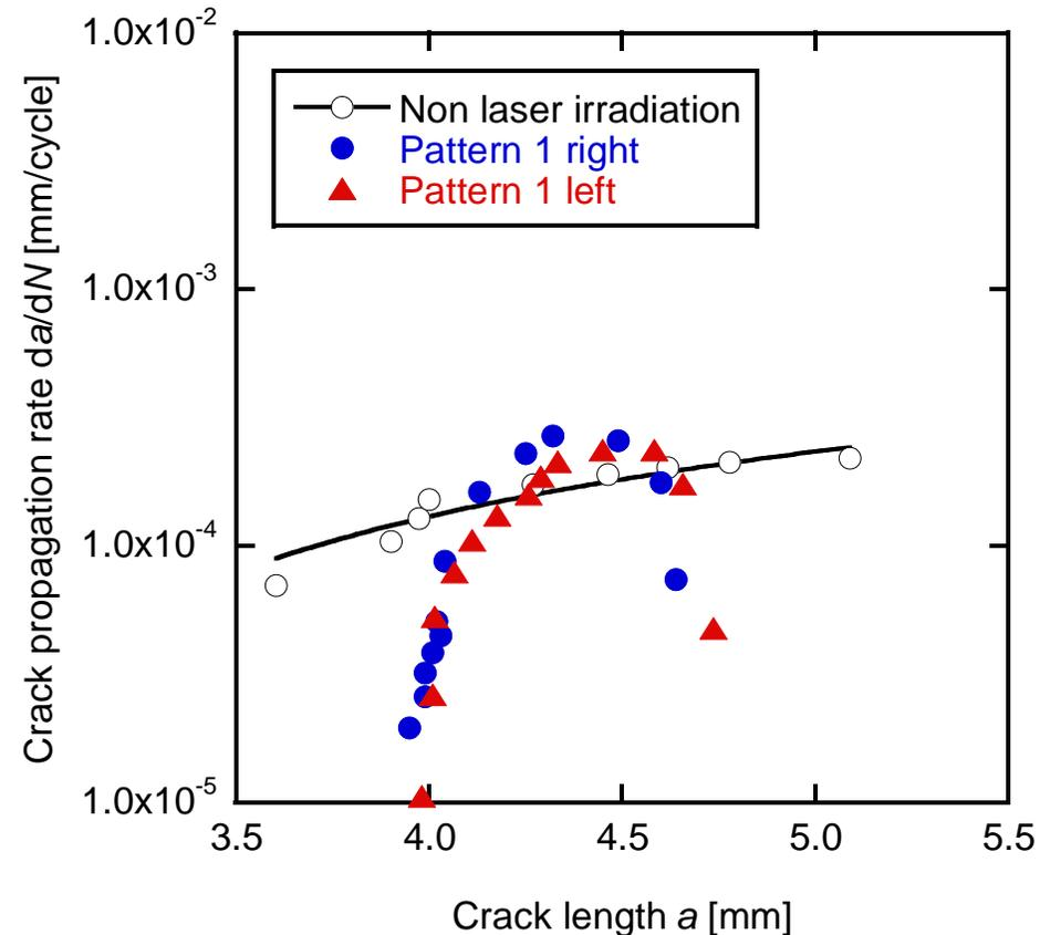
It was confirmed that crack propagation rate in crack repaired by laser irradiation was delayed in comparison with that in non laser irradiation. Thus, this technique is available for repairing small-size crack in brief process period.
