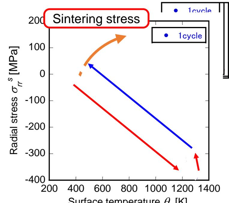
Sintering effect was taken into account in FE code. It was identified that the coating stress is increased due to sintering strain accumulation.
