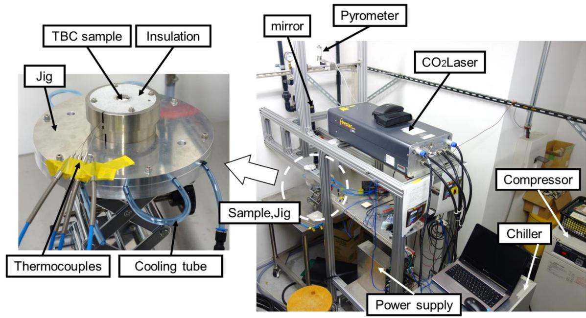
High-temperature gradient test by laser irradiation
