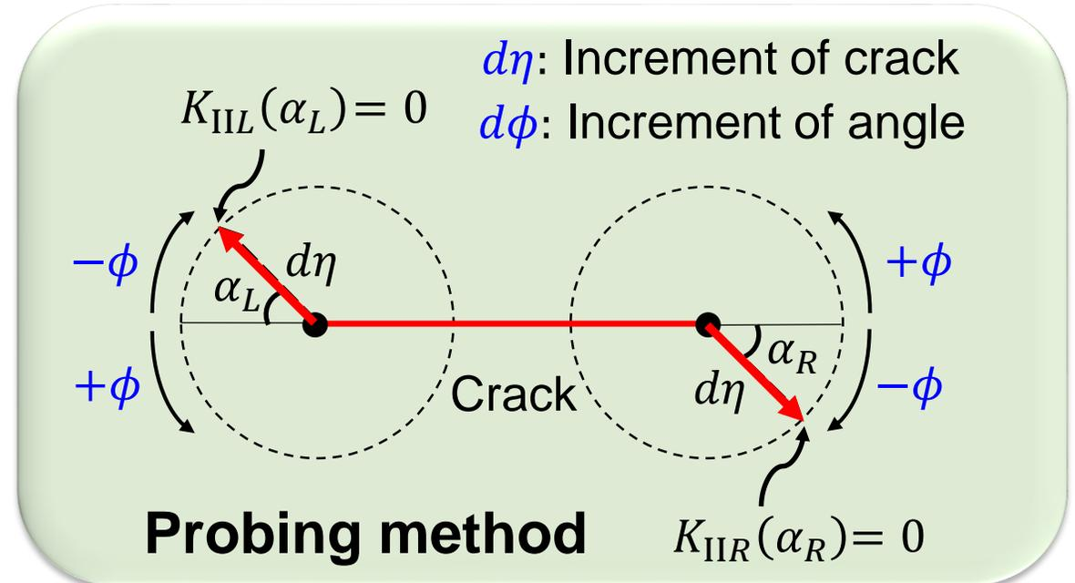
✓ Crack propagation direction
