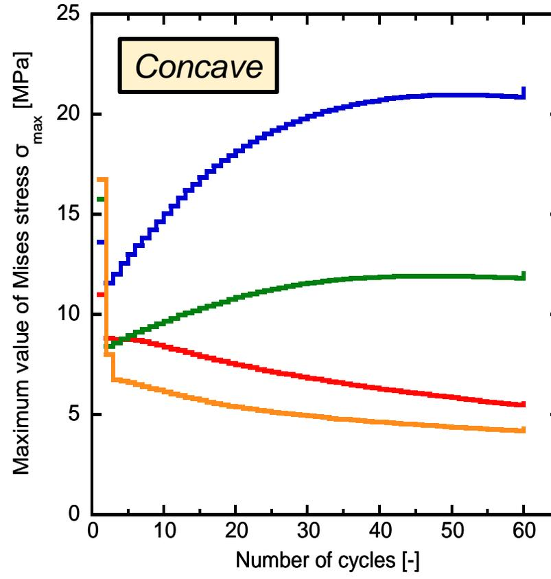
Cracks were initiated at concave in top coat, which corresponds to FE analysis.
