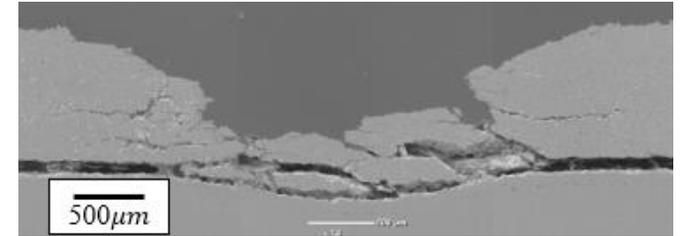
**TBC surface damage by FOD**
