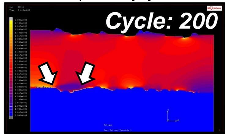
In out of phase, the interfacial crack is initiated at number of cycles shorter than one of in-phase.
