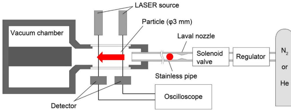
**Single Particle Impact Testing System (SPITS)**
