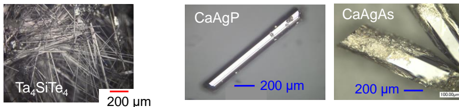
Fig. 1. Whisker crystals of \text{Ta}_4\text{SiTe}_4 . Fig. 2. Single crystals of \text{CaAgP} (left) and \text{CaAgAs} (right).
