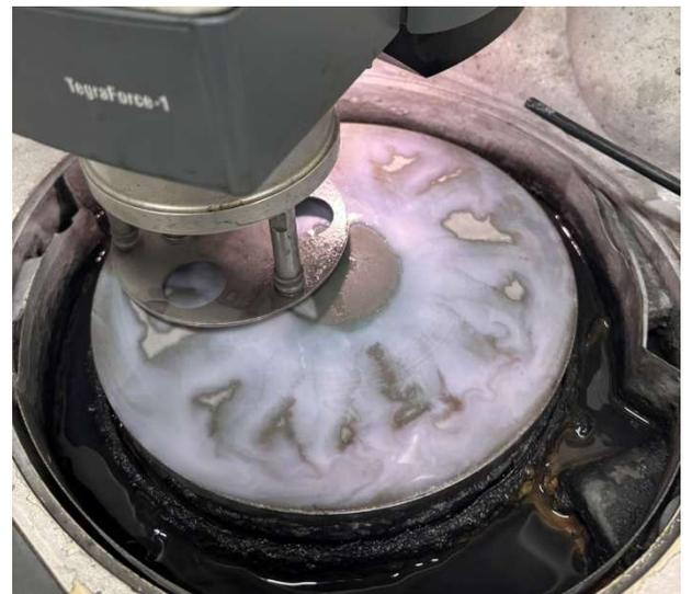
Fig. 2-4 Surface of diamond polishing
