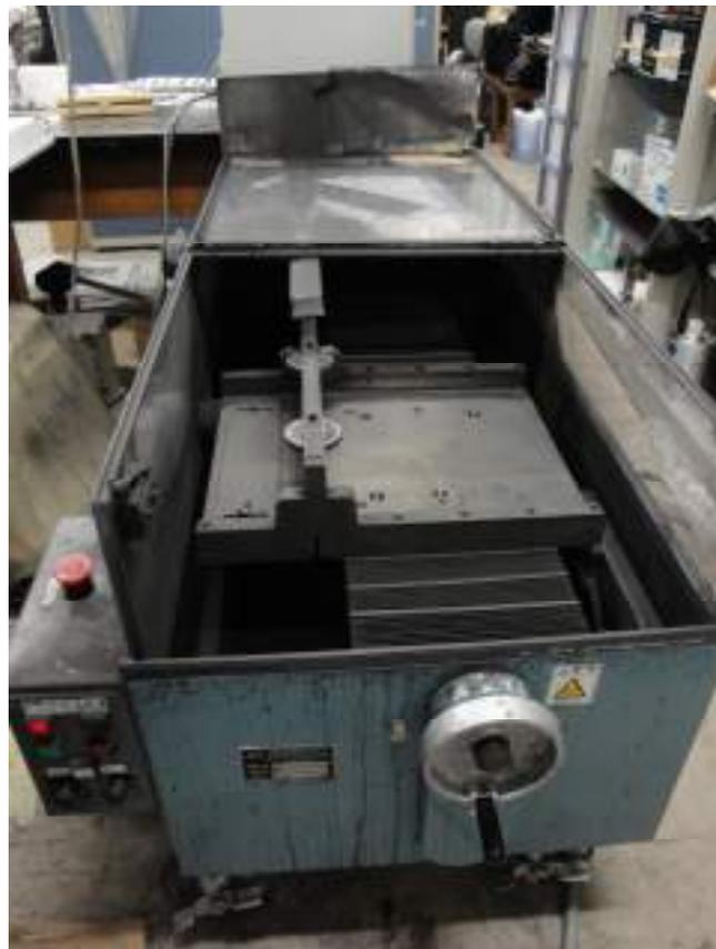
Fig. 2-1-4 Cutting machine for composite materials.
