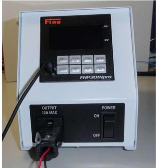
Fig.2-11 Temperature controller.
