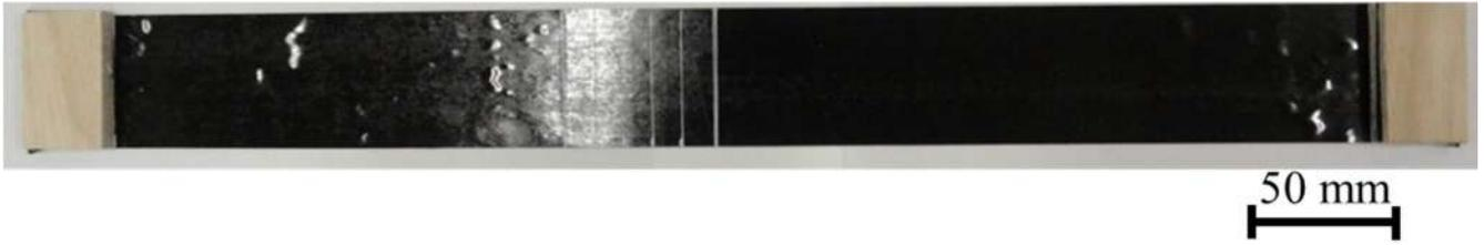
Fig.2-4 The specimen before pull-out test.
