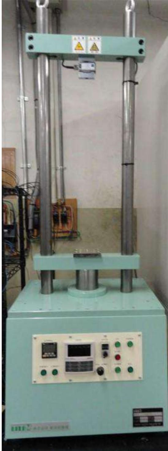
Fig. 2-8 Overview of the tensile testing machine.
